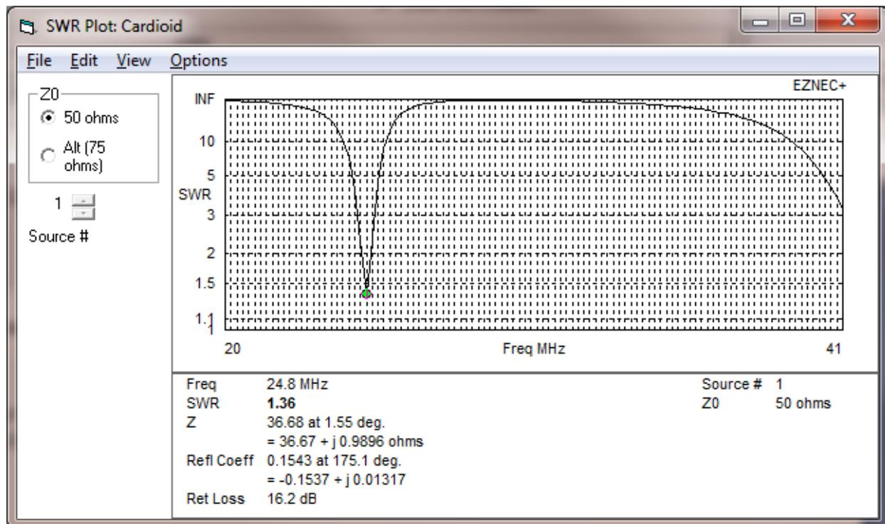
As can be seen in the above trace, EZNEC predicted that the resonant frequency of the antenna had been modified by the introduction of the transmission lines. Specifically, EZNEC indicates a resonant frequency of 24.8 MHz.
