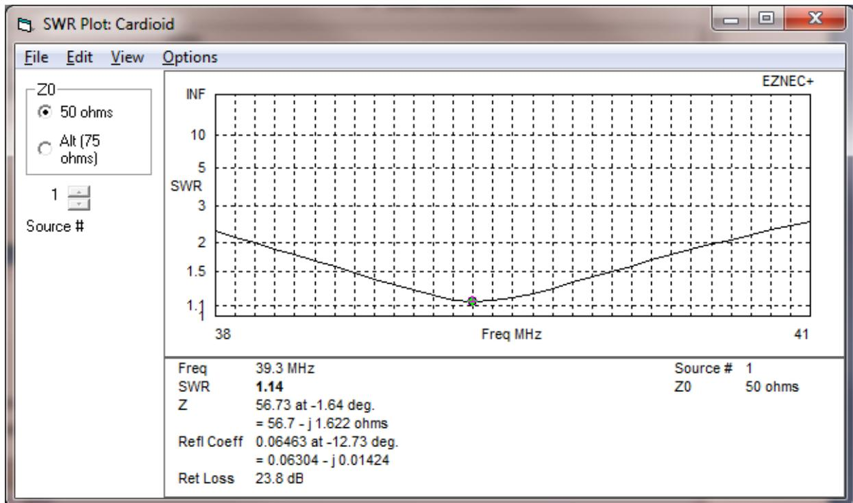
The first *measurement* I made was to find the natural frequency of the 'outer surface' of the coax. To make this measurement I connected my AIM 4170b antenna analyzer to the coax braid. I then lofted the antenna to 5 meters and ran a measurement. Here is the resulting scan:
