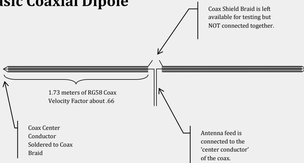
This antenna has much in common with the 'double bazooka' and my immediate 'gut feeling' was that the coax performs two functions. First, the radiating elements of the antenna would be the outer surface of the coax shield. Second, the coax segments would provide some reactance, presumably inductive, which would lower the resonant frequency of the basic dipole. In order to simplify thinking about these two functions I redraw the antenna as:
