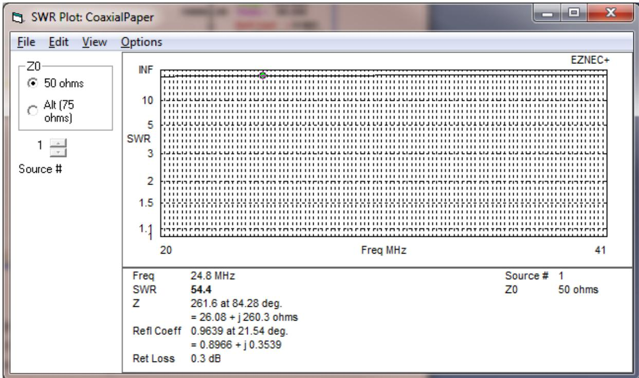
The above simulation shows the correct impedance at 24. Mhz. To get these results I had to set the coax los to 8db/100m.
