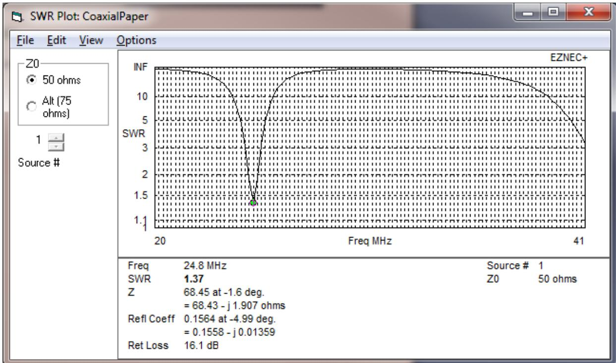
This matches VERY NICELY with the actual measurements. From these measurements and simulation I conclude that the coaxial cable operates along the lines predicted by the simplified model.
